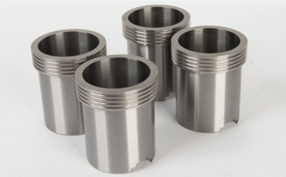
The LA Sleeve FA20 ductile iron liners retain the original open-deck design of the engine. These liners allow for a final bore of 89mm while containing cylinder pressures beyond 1,000whp.
